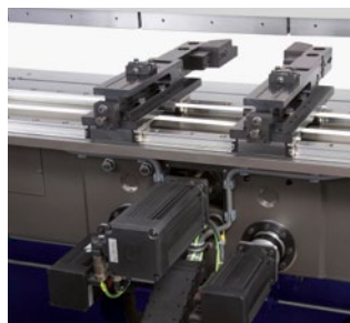
Type X, R, Z1, Z2: Four CNC-controlled axes.
